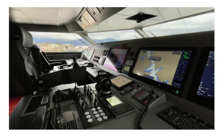
Situated atop the passenger deck, *Santa Monica* 1's wheelhouse features the latest navigation, monitoring, and control equipment. A dedicated docking station, 360-degree views and CCTV deliver a high level of safety and control during voyages and docking.
