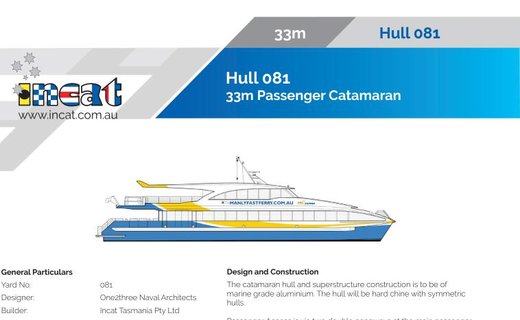
Passenger Access is via two double gangways at the main passenger level. Both main and upper decks include indoor and outdoor seating. Toilets, kiosk and surfboard and bike racks are located on the main passenger deck. Internal stairs provide access from the main deck to the upperdeck, which includes passenger areas and the wheelhouse.
