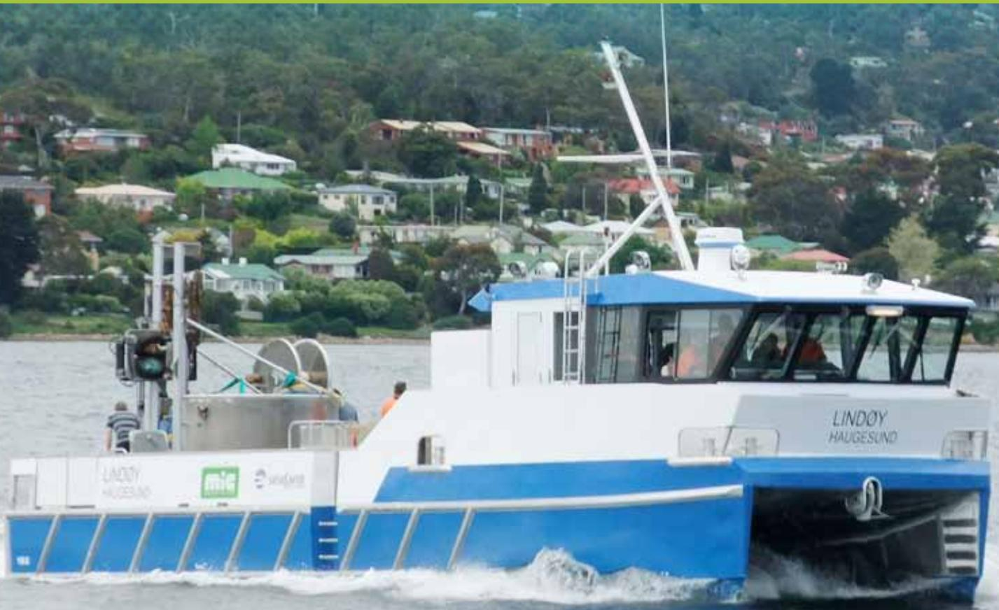
**The stability offered by the catamaran assists with station keeping while net cleaning operation is underway.**
